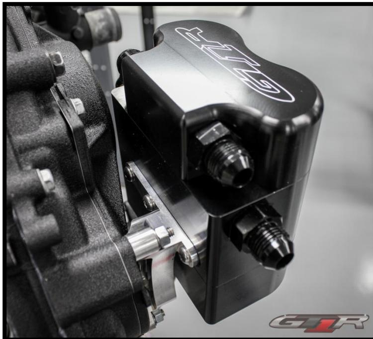
3. Install hose #8 - 15.5" 8AN hose with the 30° hose end and hose finisher on the other end. The 30° hose end goes on the bottom left port (#4) on the AOS and the other end goes on the pass side valve cover outlet.
