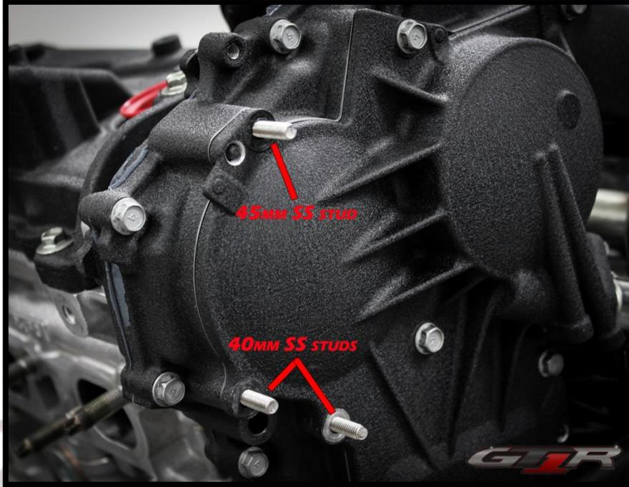
2. Install the pre-assembled AOS on the three mounting studs and install the 3 M6 nuts and washers to secure it.
