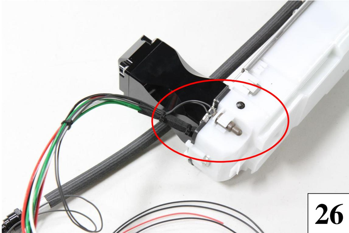
27) Route the fuel temp sensor wiring up to **Connector B**. The 2 **Black** wires of the fuel temperature sensor will need to be connected to the 2 **Black** unterminated wires on the 6 pin **Connector B**. Polarity does not matter; you can connect the black wires either way.
