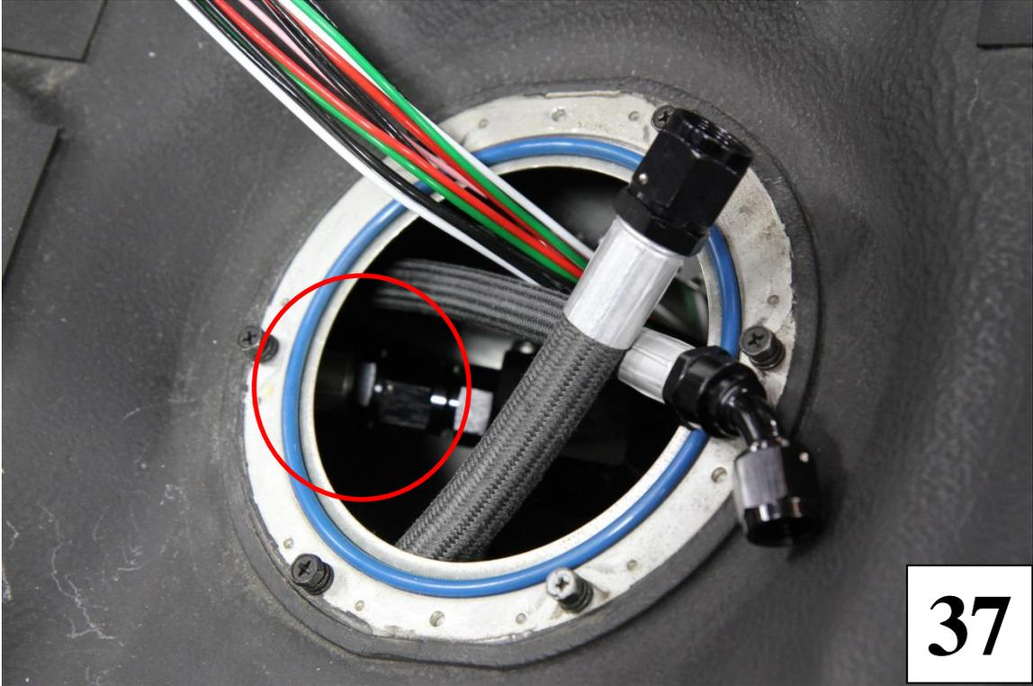
**38)** Locate the billet top hat. The Red bulkheads and fittings have already been installed for you. The electrical bulkheads are left out for now. They are the last piece to be install once the billet top hat is final installed.
