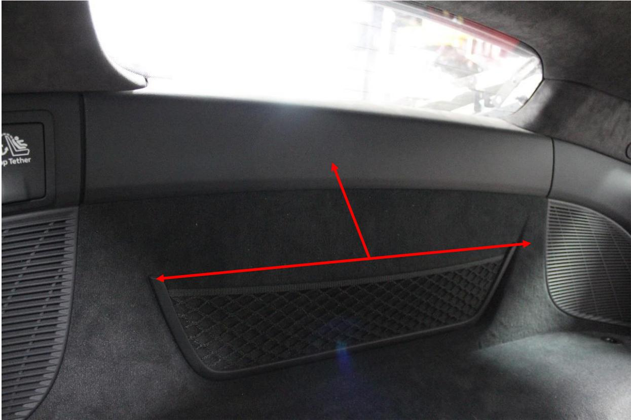
5. Remove the plastic screw under the speaker grille on each side.
