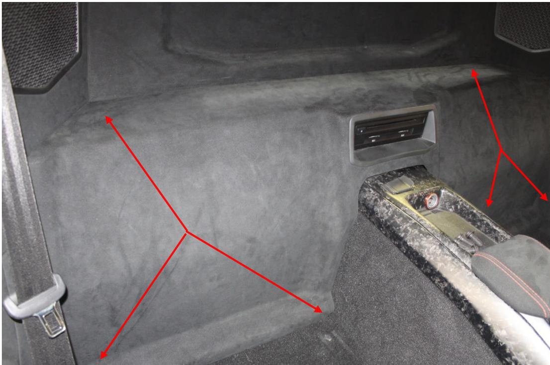
8. Remove the panel between the headliner and window trim.
