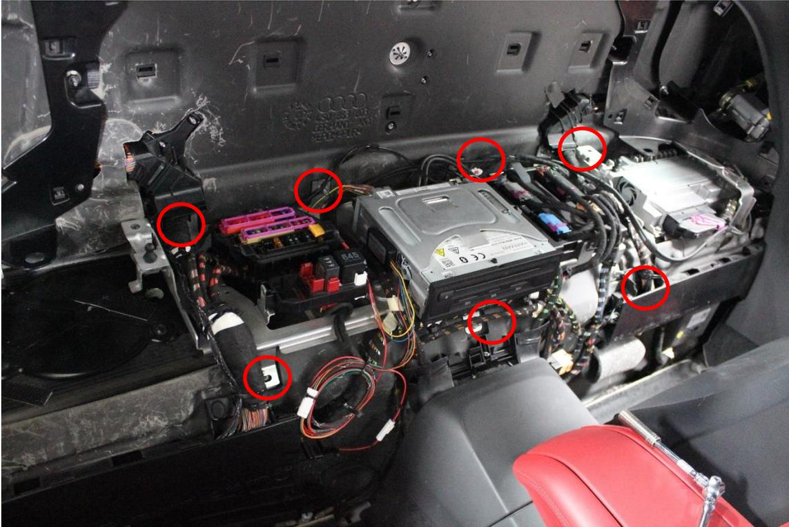
12. Pull the bracket assembly towards the front of the car to release it off the studs. I found propping it up with a block of wood to be helpful to remove the access panel.
