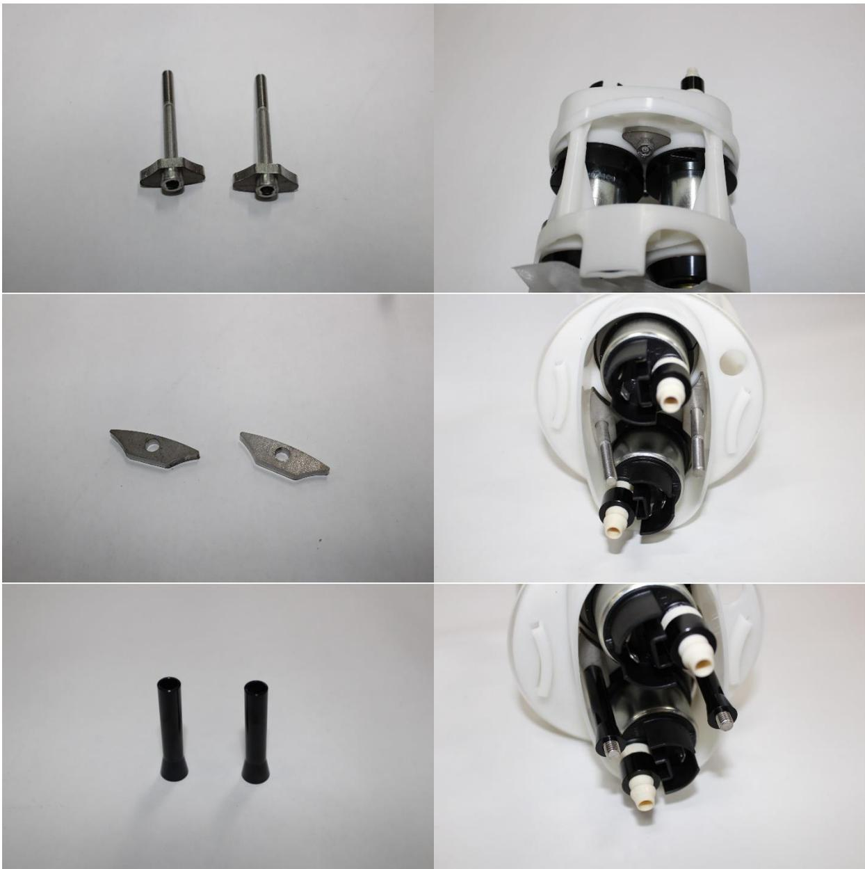
32. Lubricate the grommets in the fuel pump manifold and install onto the pump bars. Notice the orientation of the manifold in reference to the basket. Then tighten the allen bolts.
