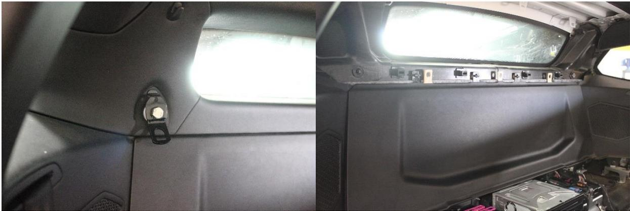
10. Remove the four nuts holding the lower panel and remove the panel.
