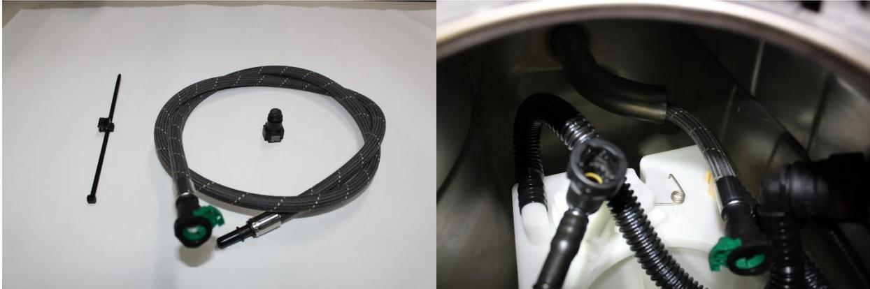
37. On the driver side tank, route the line away from the level sensor by leaving a little slack in the line and wrapping around the backside of the sensor with the zip tie mount. Then make the connection as shown in the last photo below.
