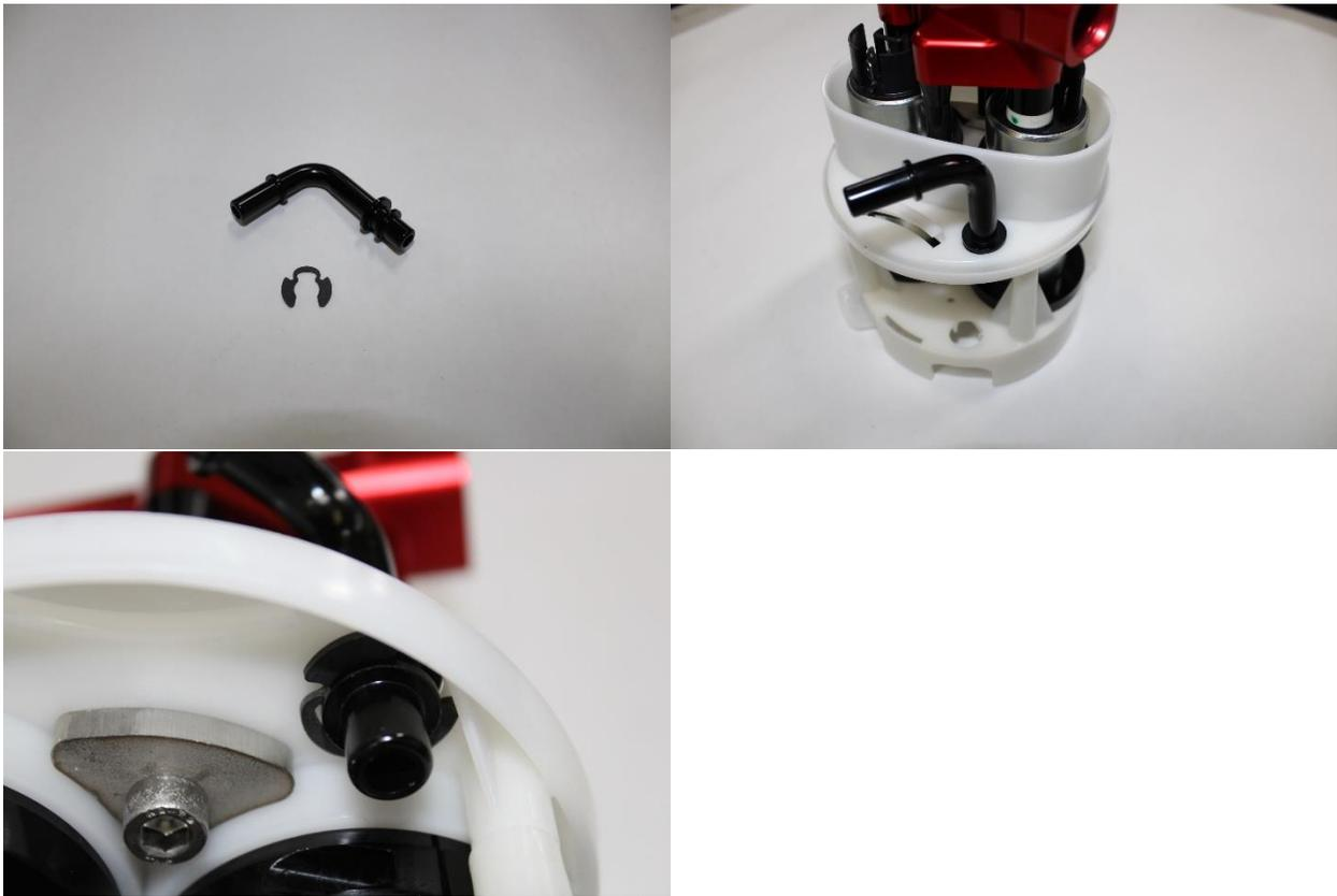
34. Using the provided M4 bolts, Snuggly fasten them into the top cap to hold the pumps in place. Do not overtighten them as you may damage the pumps. Then set it aside for now.
