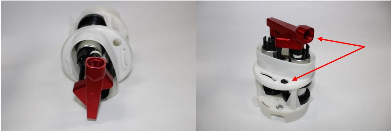
33. Locate the black fuel return fitting and retaining clip. Install the fitting into the hole drilled in step 24. Install the retaining clip on the backside.
