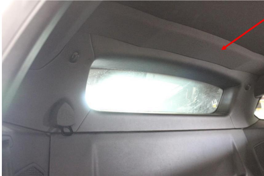
9. Remove the plastic cover to reveal the bolt holding the child seat hook. Then remove the window trim plastic.
