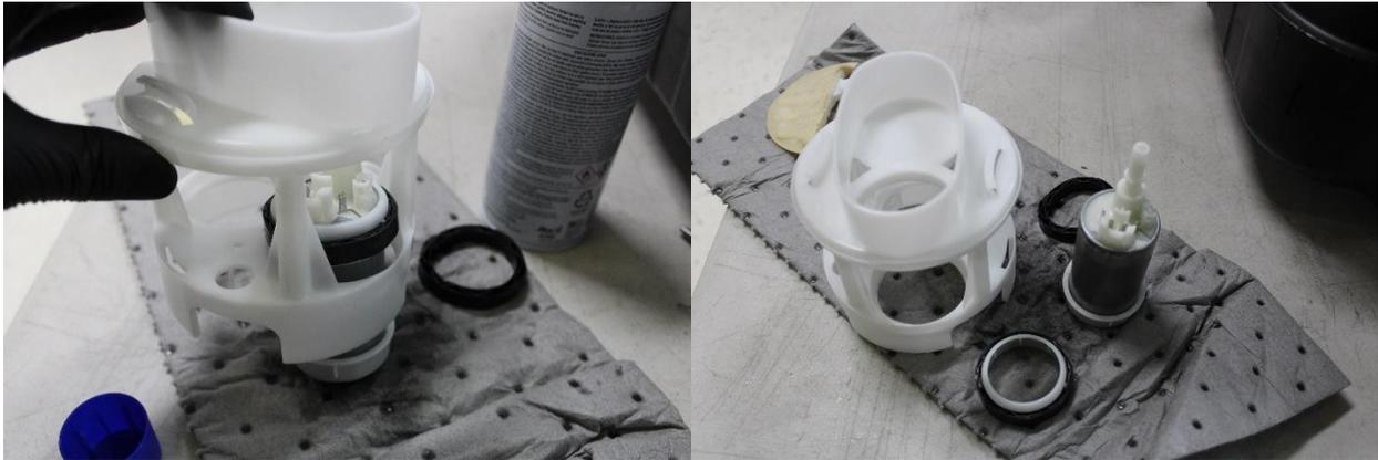
24. Using the empty basket, locate the 3D printed drill jig and set it in the top of the basket in such a way it covers the open hole. This will locate the holes to be drilled. Using a 2" hole saw and a 14mm (or similar) drill bit, drill the two holes as shown below. Remove any burrs or debris.
