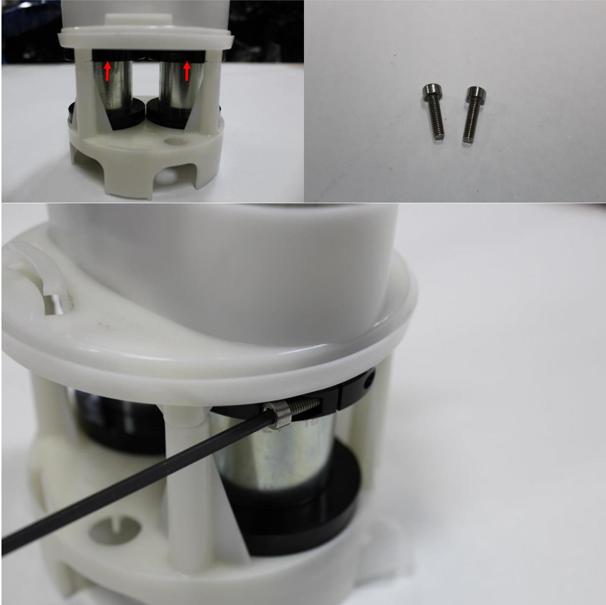
35. Next, we need to make a few changes to the driver's side tank for the Alpha Dual Brushless Fuel System. Start by removing the access panel and fuel tank retaining nut as you did before. Locate the fuel filter/fuel pressure regulator assembly near the back of the tank. Release the quick connect fitting and the strap holding the assembly. Then remove the assembly.
