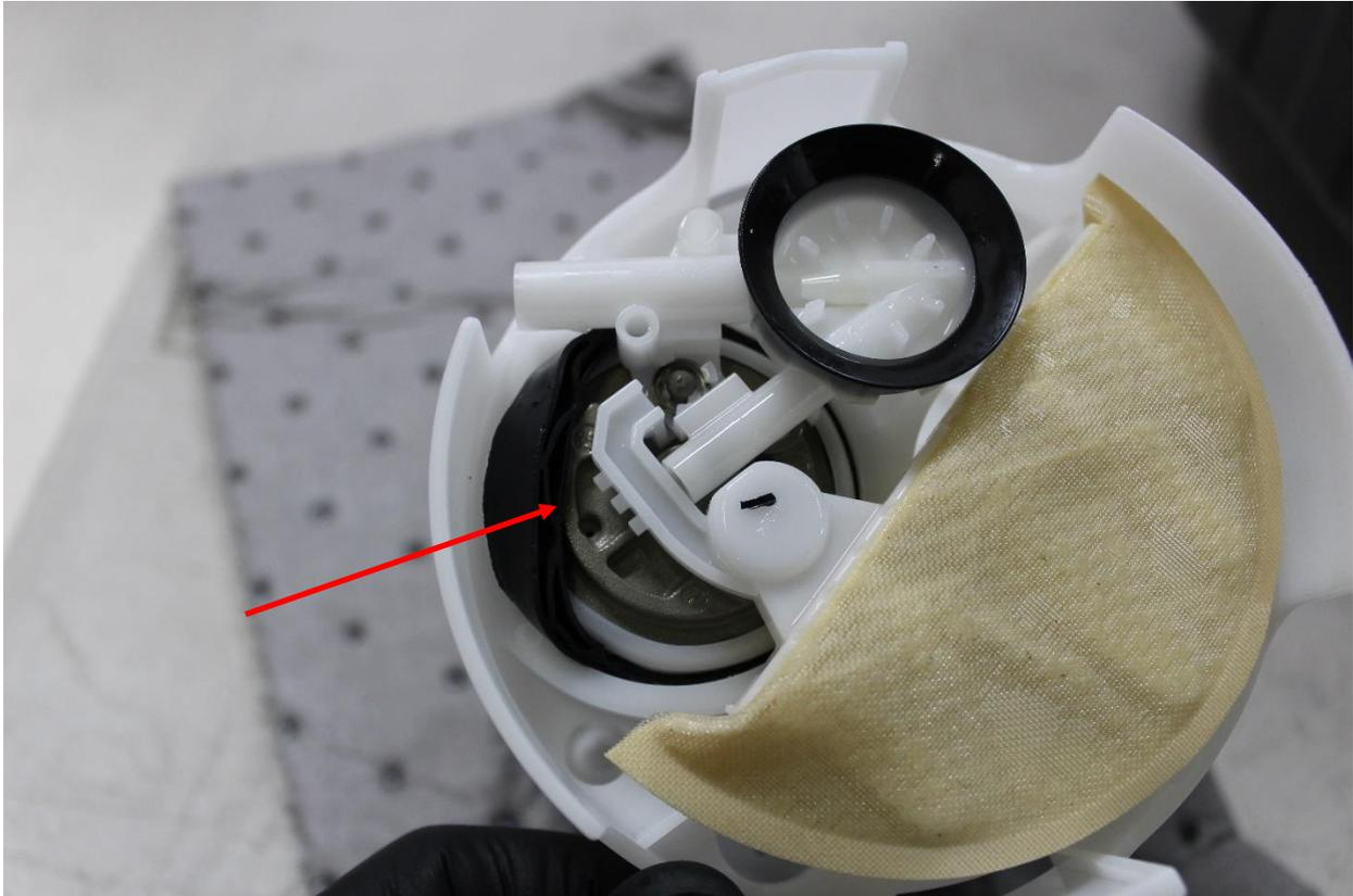
23. Remove the entire rubber spacer and the pump should drop out. Remove the rest of the parts so you are left with a bare basket.
