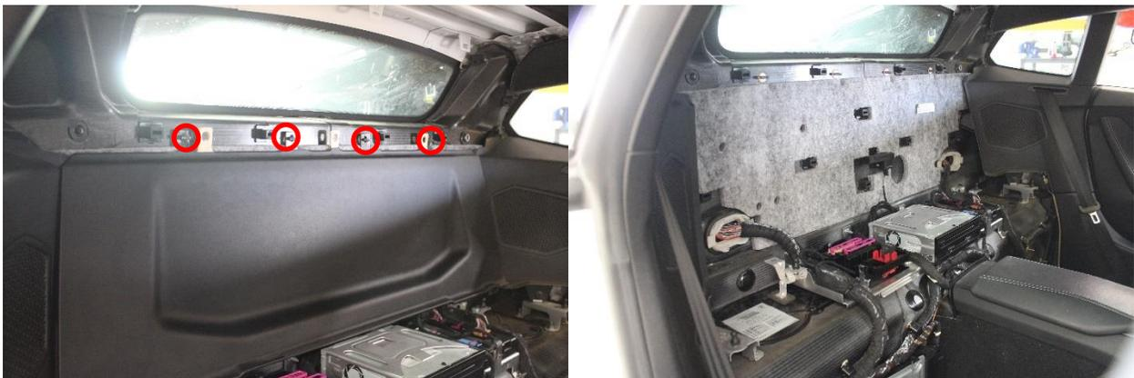
11. Remove the seven nuts from the control unit bracket assembly to gain access to the fuel tank access panel bolts.
