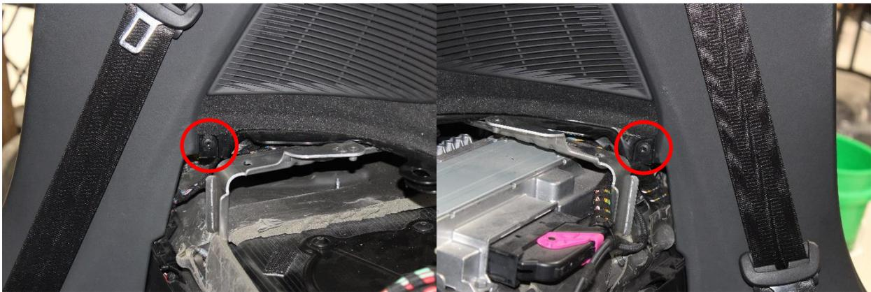
6. Remove the four nuts along the top of the rear trim panel.
