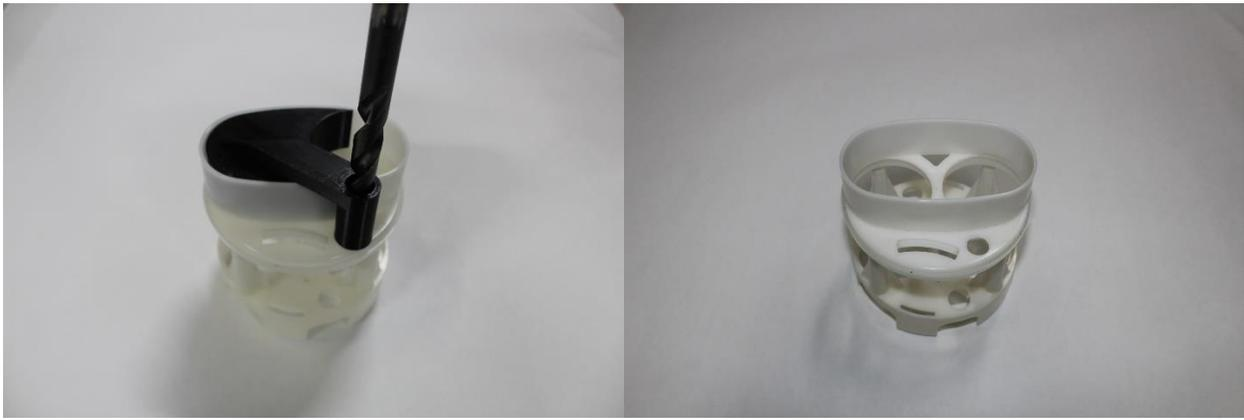
25. Gather the following parts – fuel pumps, filter pickups, O-rings and top & bottom caps. Starting with the top & bottom caps, notice two have a section machined out to create a light cinch feature (top cap) while two do not (bottom cap). Grab one of each and place an O-ring inside the groove as shown. This will be for the first pump.
