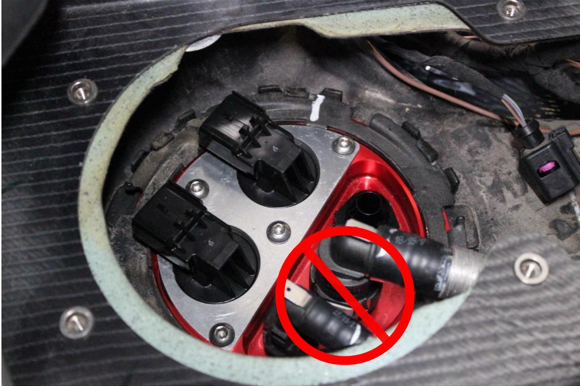
52. Now you can install a new seal (provided) to driver's side tank. Then reinstall the factory top hat, top hat nut and connections.
